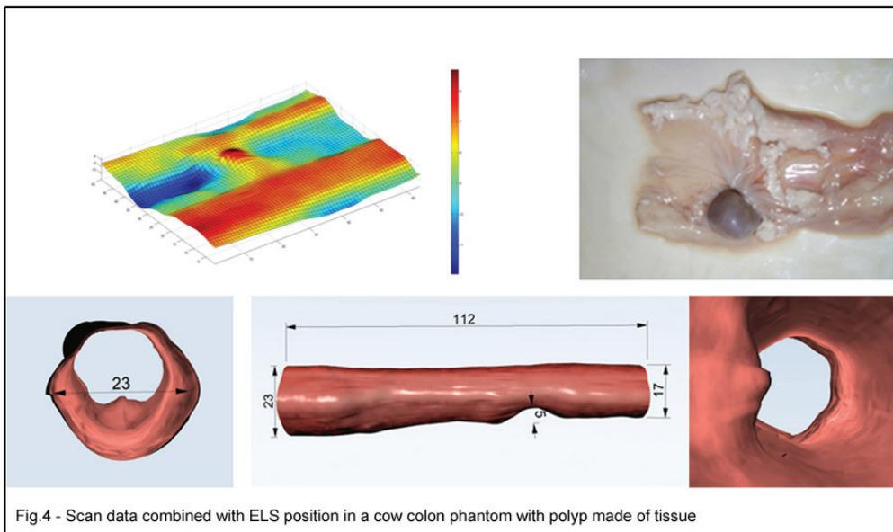
Fig.4 - Scan data combined with ELS position in a cow colon phantom with polyp made of tissue
