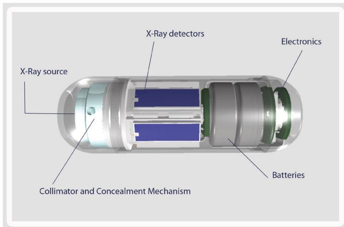
10 capsules were swallowed by volunteers M=7 (ages 37 - 66) and were tracked during the whole passage of the capsule in the body using radio frequency telemetry and an Electromagnetic Localization System (ELS). The capsules were programed to perform scans when movement in the colon is detected and transmit the imaging data to an external recorder unit worn by the patients. The study was approved by the IRB of the Tel Aviv Medical Center.
